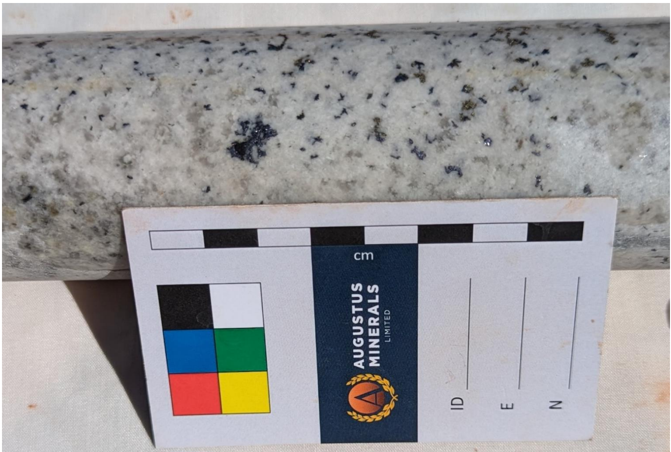
Figure 2 Disseminated molybdenite (silver) within MSD010 at 248.28m within interval 248.15m to 248.71m (0.56m) which averaged 2% molybdenite and 1% pyrite.
