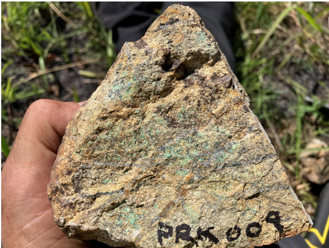
Figure 9 Copper stained (malachite) in strongly quartz stockworked intrusive. Grab sample estimated to assay ~0.5% Cu and ~1g/t Au. Peenam prospect October 2024
