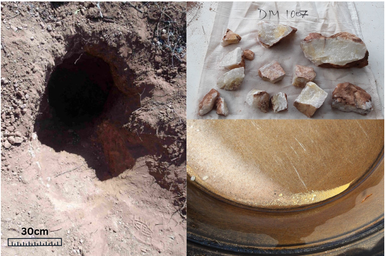
Figure 2. Sample DM1007 @ 2,040g/t Au. Hole from where DYM1007 was taken (left), quartz sample sent to lab (top right) and gold panned from dollied sample in the field
