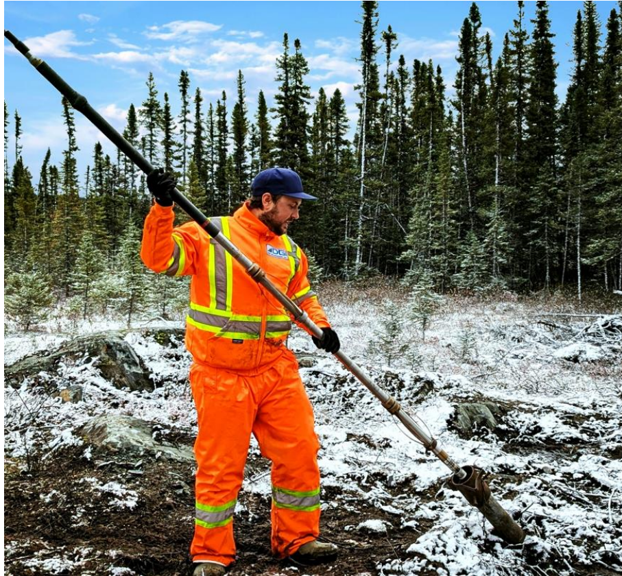
Figure 12: Televiwer survey instrument being placed in drill hole CV24-492.
