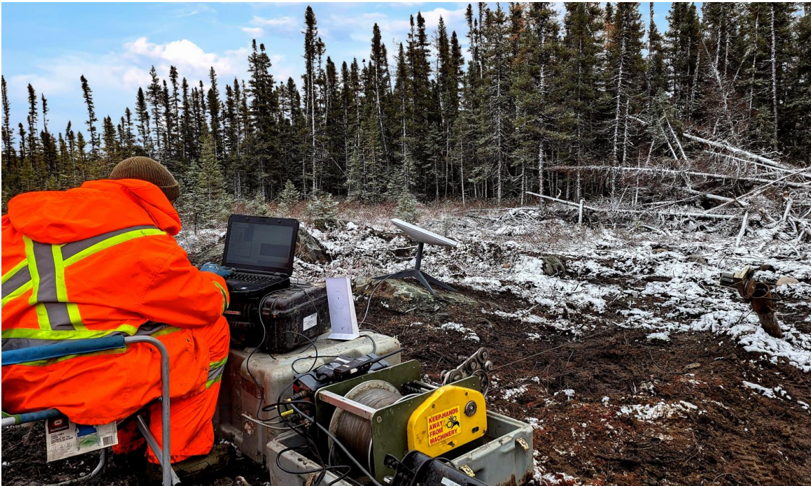
Figure 13: Televiwer survey data collection in drill hole CV24-492.
