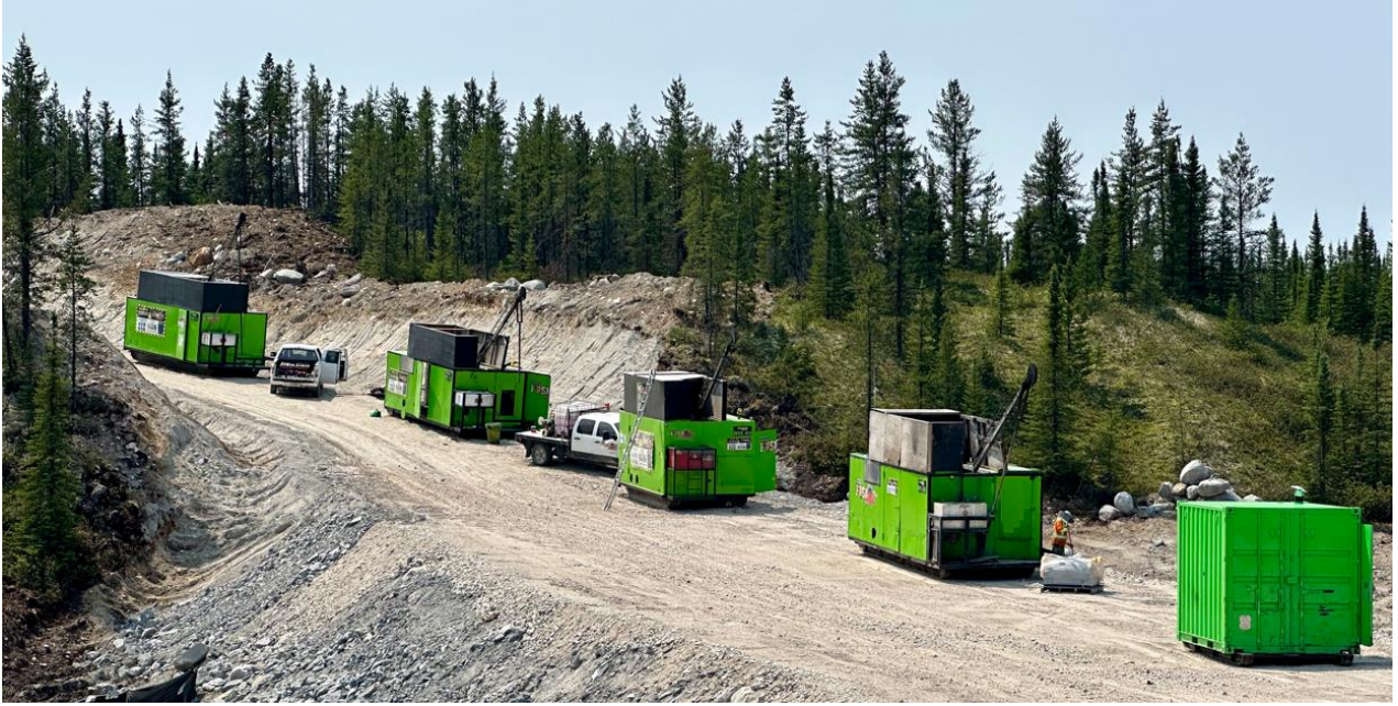
Figure 3: Four skid-mounted drill rigs ready for deployment to the southwest area of CV5 using the Company's all-season road. No helicopter support required.
