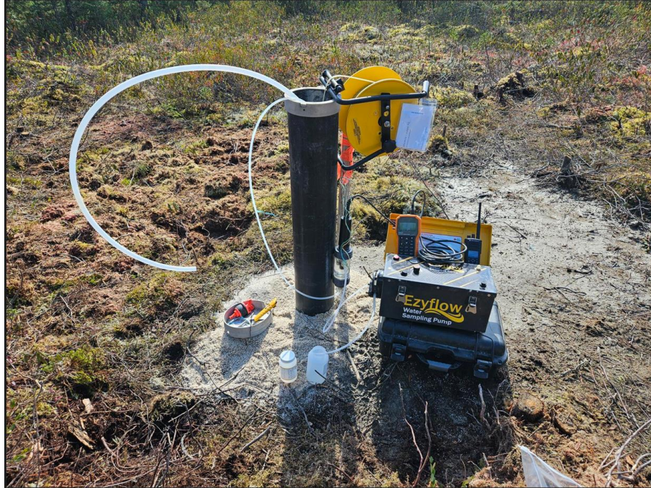
Figure 9: Monitoring well installation in drill hole CV24-672, situated north of CV5.
