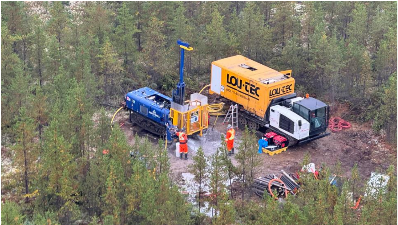
Figure 10: Drill hole CV24-696 (6-inch diameter) completed at CV5 for long-duration pump test to assess pit dewatering.
