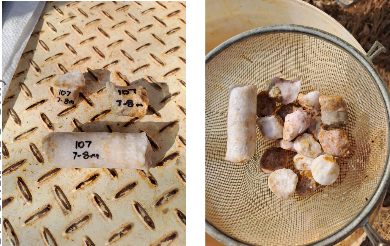
Figure 4: Quartz veining consistent with known mineralisation styles from the Northern and Central Targets on the Alice River Project, recovered from Aircore drillhole ARAC-107 1 .
