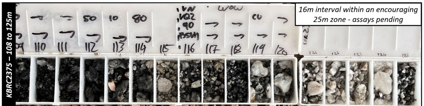
Figure 13: KBRC2375 chip tray 109 to 125m, 25m down dip of KBRC2302 (above) showing potential widening of sulphidic shale (pyrite, chalcopyrite, malachite, molybdenite & sphalerite), brecciated quartz and carbonates.
