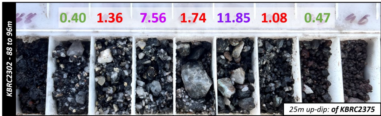
Figure 12: KBRC2302 chip tray 88 to 96m ore zone consisting of sulphidic shale (pyrite, chalcopyrite, malachite, molybdenite & sphalerite), brecciated quartz and carbonates, with Au ppm assay results top.
