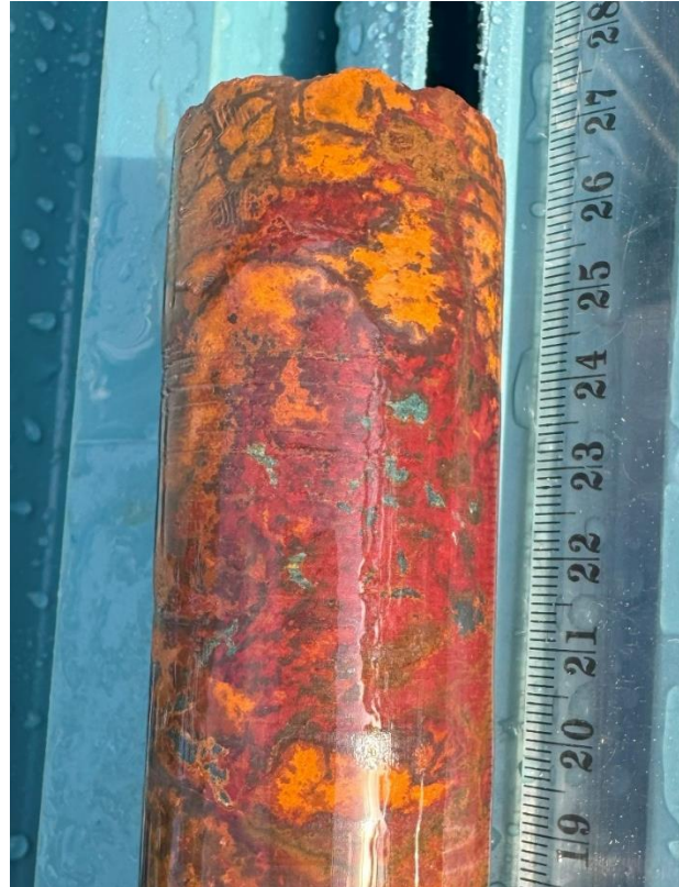
Figure 2: Copper (malachite blebs with chalcocite rims and chalcocite blebs) in oxidised dolomite/ankerite host vein of Hole WYPC04 at Worrumba 22.
