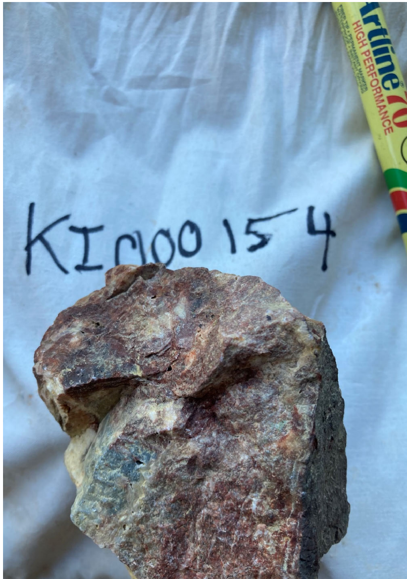
Figure 3: Rock chip sample KI000154 with a gold assay of 3.5g/t for the Mustang Prospect, note the vuggy texture in the quartz host.
