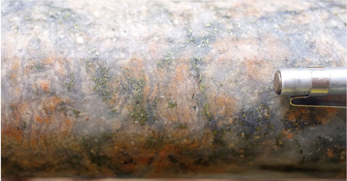
Figure 5. Strongly silicified and altered Briggs granodiorite with micro-UST textures and extensive copper sulphides. Hole 24BRD0026 at 40.5m, from a 2m interval which assayed 1.55% Cu.
