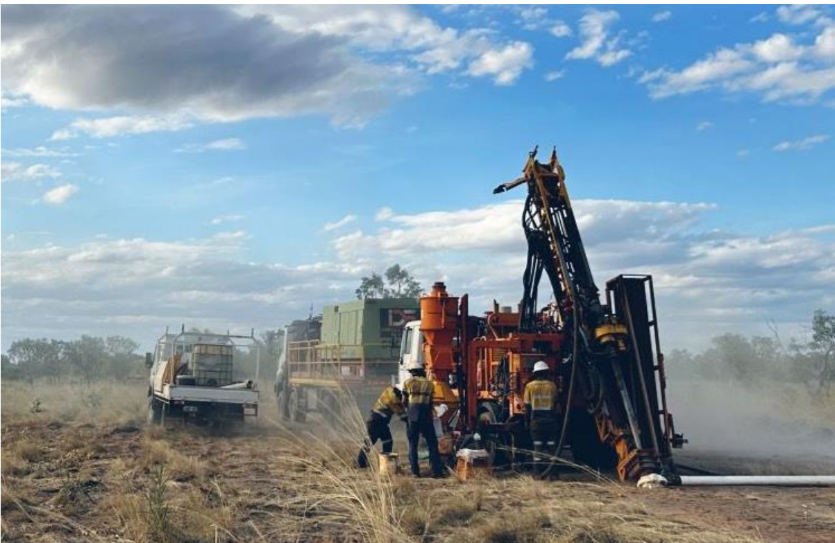
Figure 2: Drilling in action at the Christmas Creek Project. Impact Drilling's slim-line RC rig at the Martin Prospect in August.
