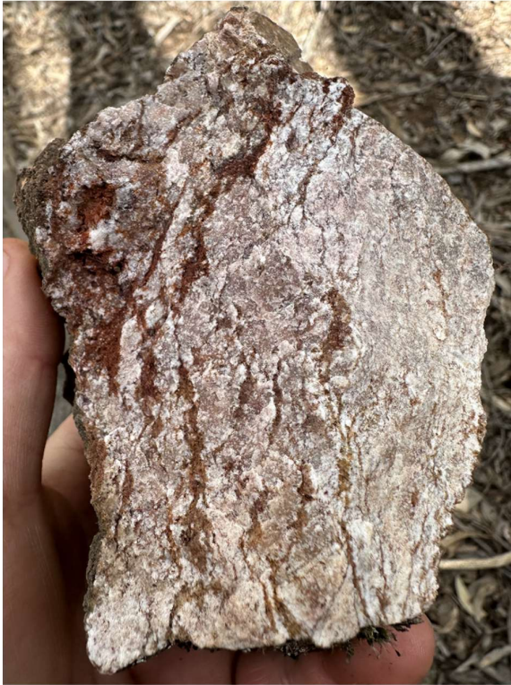
Figure 4 – Silver-Base metal mineralisation within ferruginous baritic sandstone yielding 126 g/t Ag, 0.23 g/t Au & 0.73% Ba from sample 3000937
