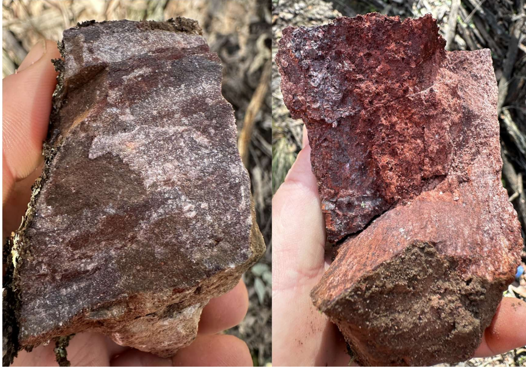
Figure 1 – Silver mineralisation within ferruginous barite outcrop yielding 117 g/t Ag , & 0.26% Ba from sample 3001009
