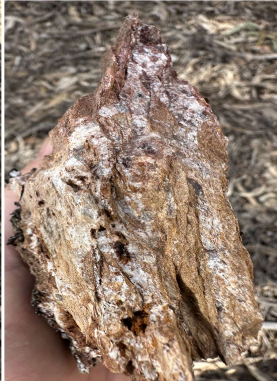
Figure 5 – Gold-Silver-Lead mineralisation within ferruginous siltstone with sulphide clast yielding 2.45 g/t Au, 13.5 g/t Ag, 0.14% Pb & 0.66% Ba from sample 3000940
