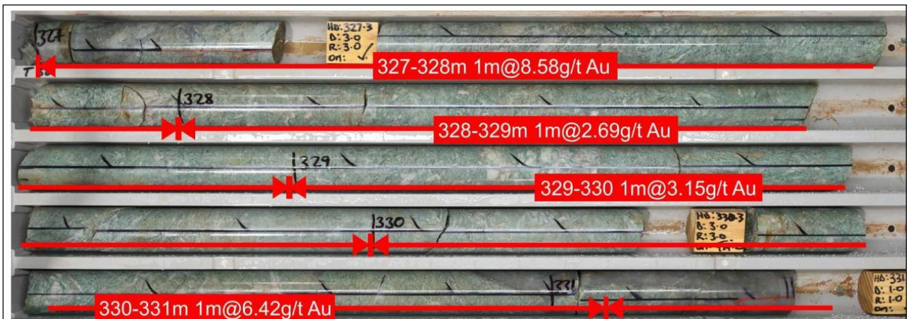
MLJDD042 Silicified ultramafic with fuchsite Alteration
