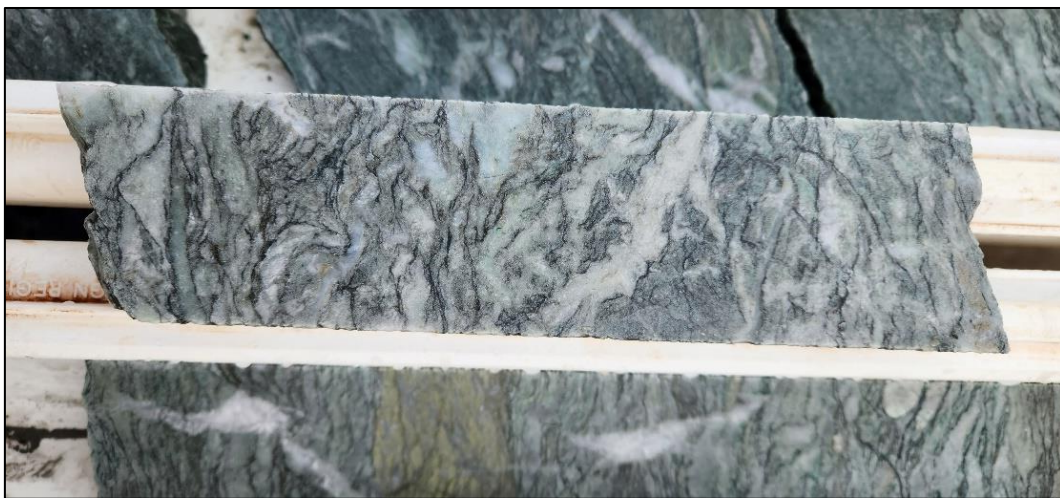
Figure 11. Drillhole MLJDD019 from 148.4m showing visceral texture in bleached, silicified ultramafic
