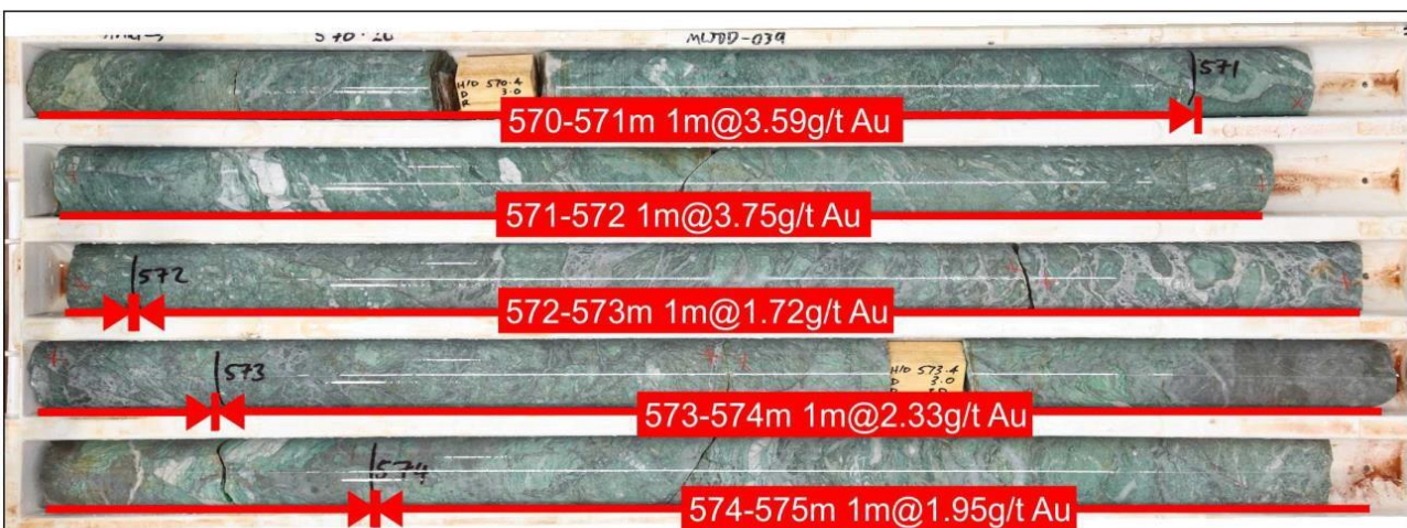
MLJDD039 Silicified ultramafic with fuchsite Alteration
