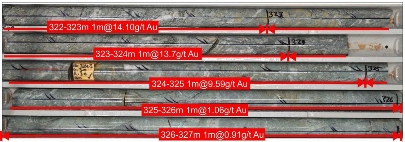
MLJDD042 Silicified ultramafic with fuchsite Alteration
