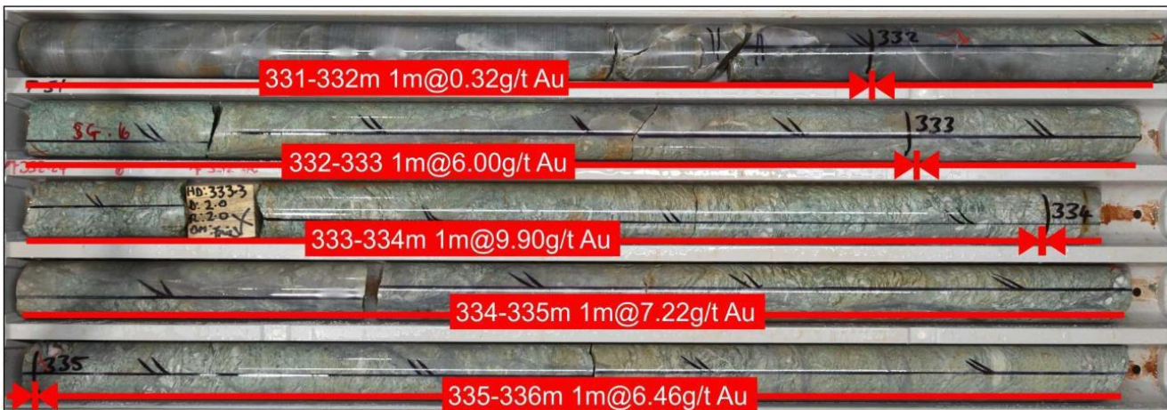
MLJDD042 Silicified ultramafic with fuchsite Alteration
