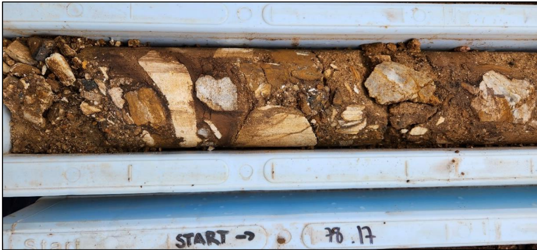
Figure 7. Drillhole MLJDD018 from 77.5m showing Polymictic Breccia
