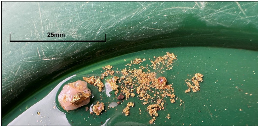
Figure 2: YMRC077 pan sample showing abundant fine and coarse gold associated with quartz veining for the interval from 51-53m which returned: 2m @ 101.50 g/t Au from 51m downhole depth
