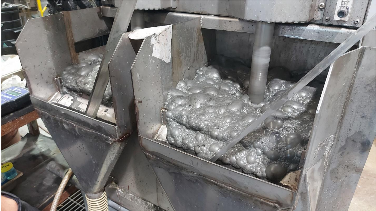
Figure 3: Photo showing sulphide flotation testwork being undertaken on the non-magnetic tail.
