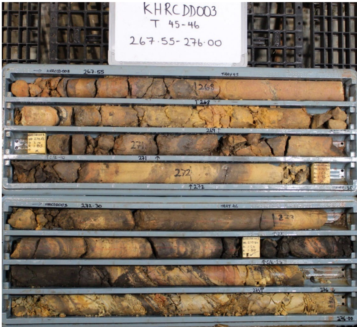
Figure 4: Ferruginous-gossanous oxidised Preston Formation sediments, KHRCDD003. Refer to Table 1 for assay grades.
