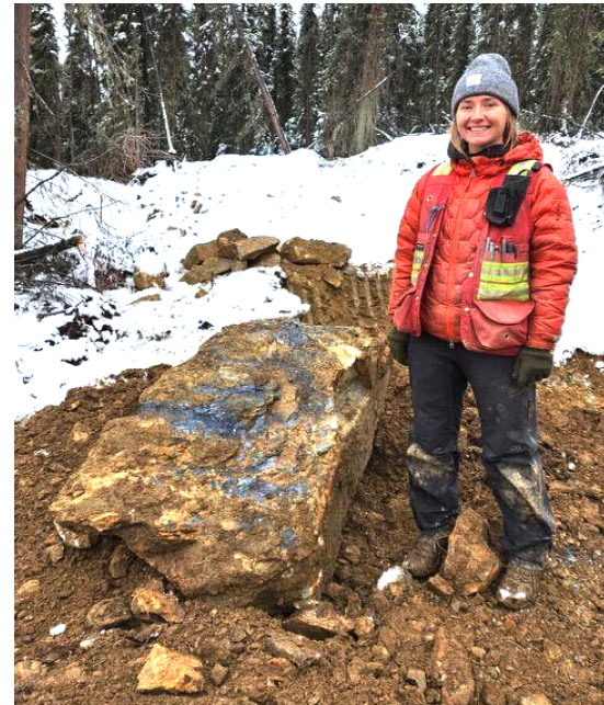
Fig. 1: Stibnite uncovered in trenching at NW Array
