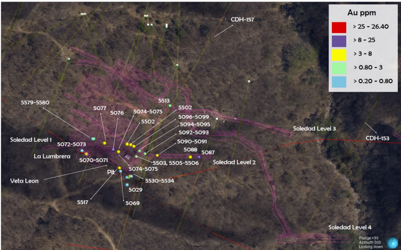
Figure 3 La Soledad workings underground channel sampling (Target 1 area)
