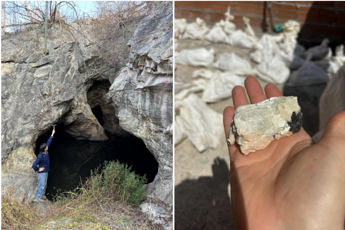
Figures 8 & 9 - Artisanal mine (left) & Spodumene with Orthoclase & Tourmaline located from within artisanal mine (right) from Isabella Project, license 830167/2013, (Refer to ASX Appendix 1 for full rock descriptions) 10
