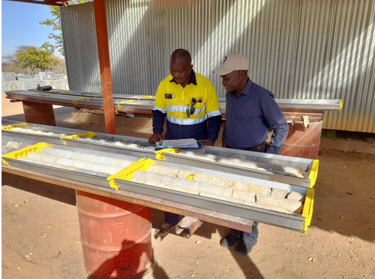
Figure 3: Lotus Resources geologists examining PQ sized diamond drill core from Serule West at the company's core storage yard.
