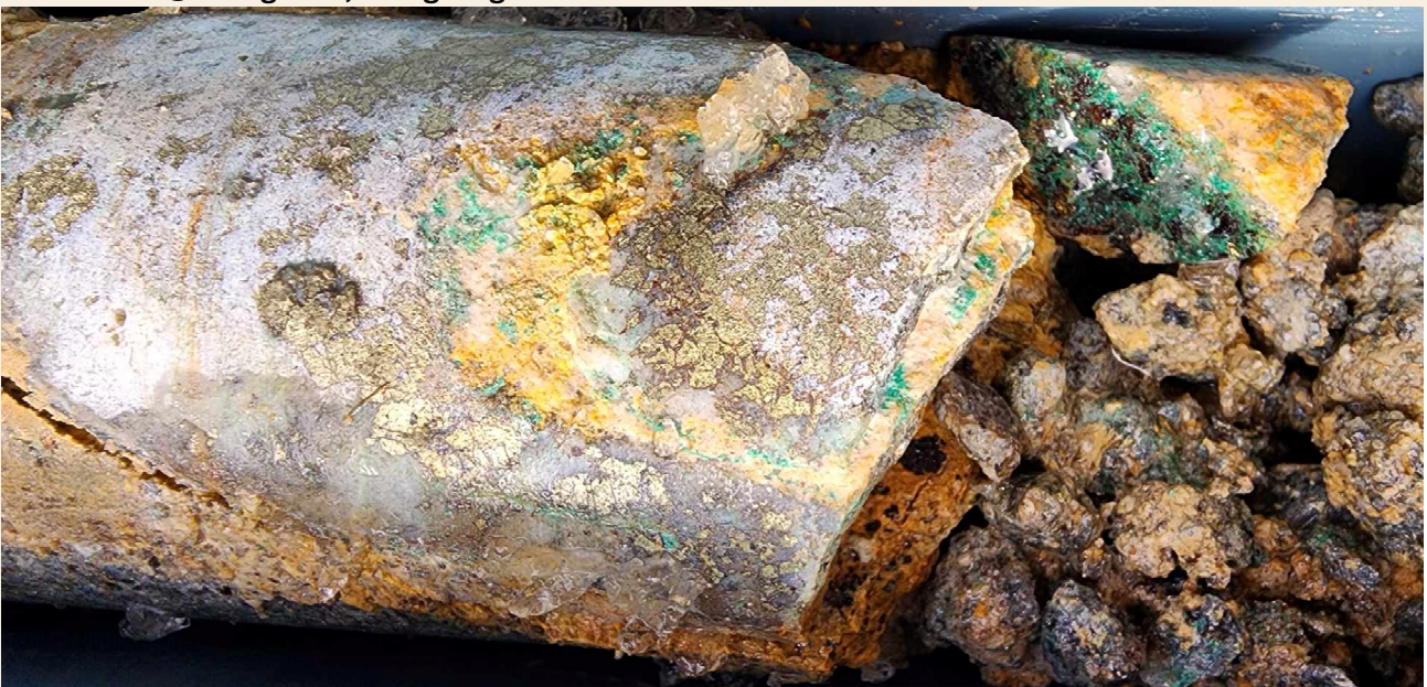
Figure 1. MRDD003 at 23.9m quartz vein with visible malachite and chalcopyrite, and goethite after sulphides, returning 0.5m @ 0.24g/t Au , 40.8g/t Ag & 3.7% Cu in assay.
