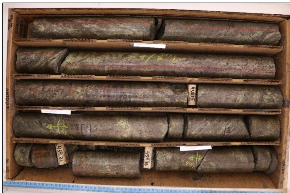
Figure 1. ANT137 Massive Sulphide Mineralisation (436.55m to 439.67m)
