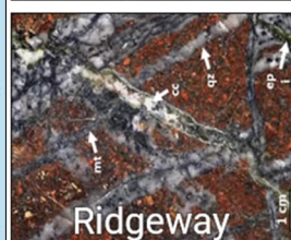
Core samples from the Rockley Prospect showing similar alteration/veining to Cadia and Ridgeway
