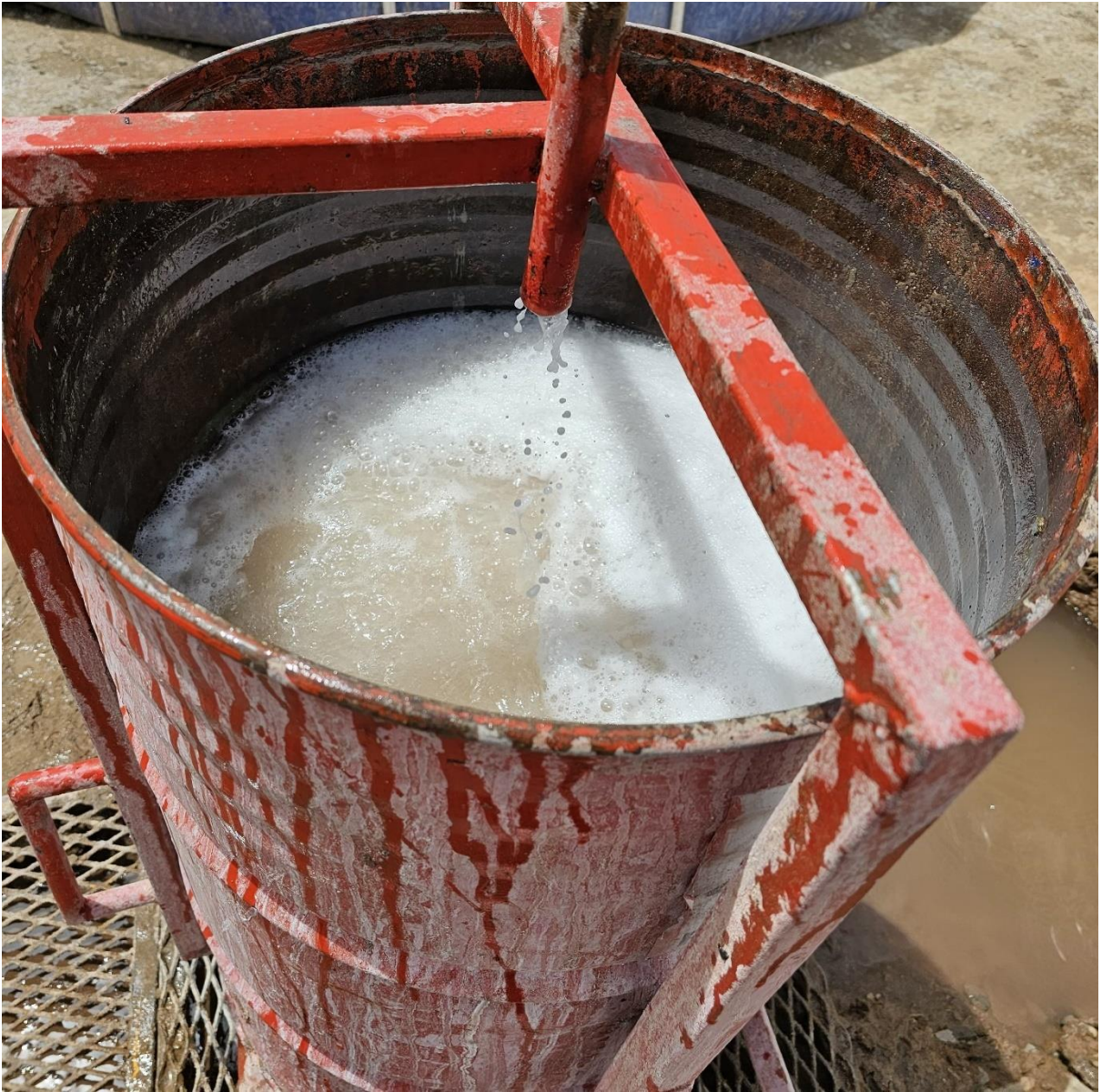
Figure 1. brines being pumped into 200L tank for assay during packer test.
