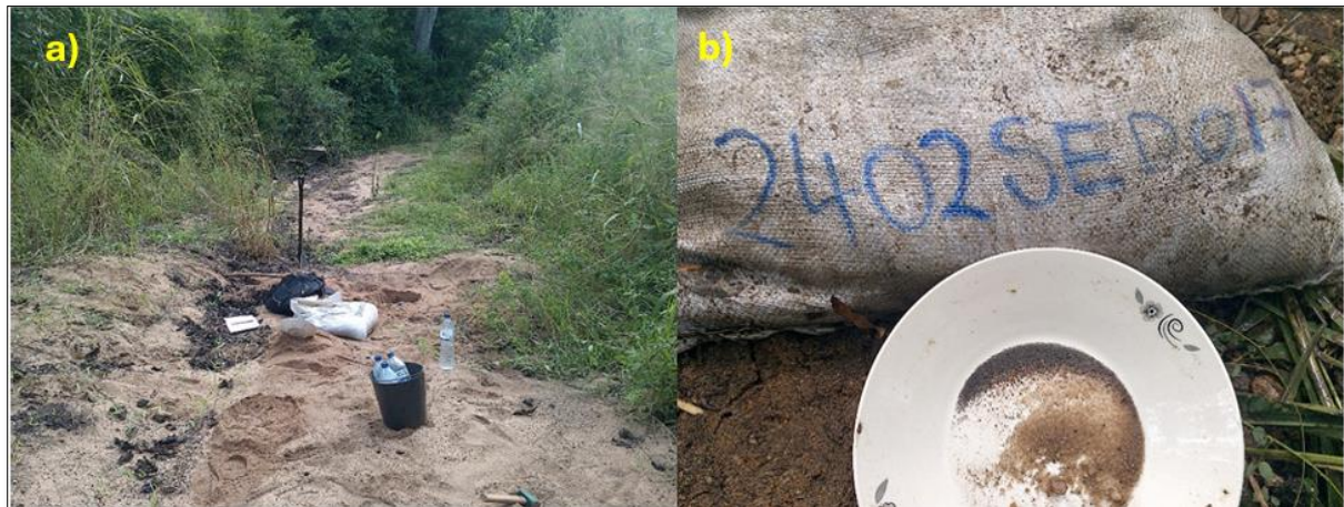
Figure 9: a) typical stream sediment sample location and equipment in the field at Adriano 11002L; b) sample 2402SED017 in the field, one of the samples with very high TREO results as seen in the pan.
