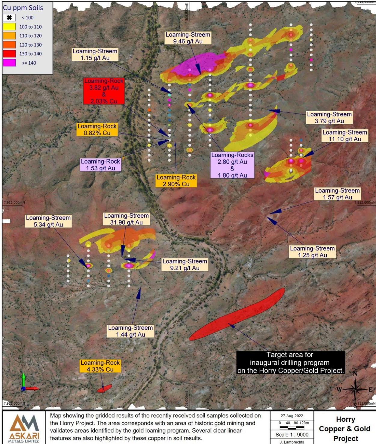
Figure 8: Gridded copper in soil results from the Horry Project
