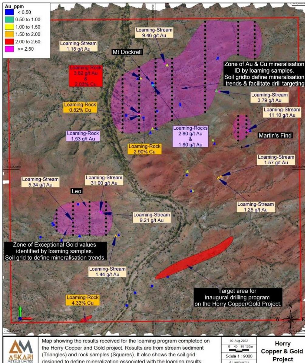
**Figure 5:** Map of the stream and rock sample results collected during the loaming survey. The location of the soil sampling program is also indicated
