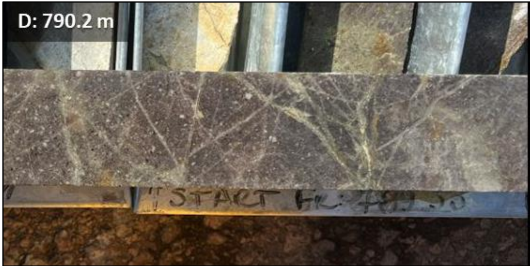
Figure 5. Core photo showing D vein stockworks in potassic-altered porphyry, from 792m depth in ZRJD23001.
