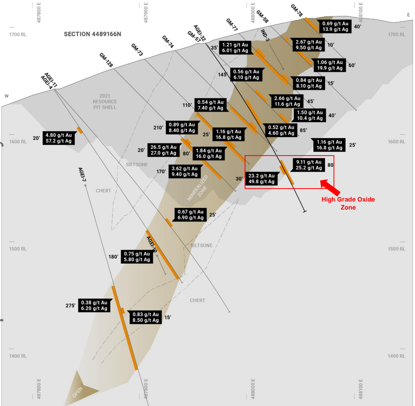
Figure 1 – Near-surface cross-section with high-grade oxide zone (within red box currently outside the existing NI 43-101 Mineral Resource).
