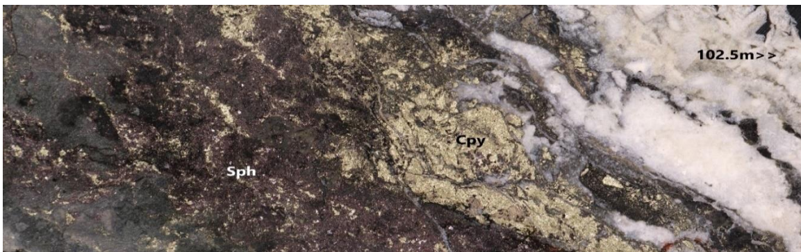
Image 1: HVD003, 102.3 - 102.5m semi-massive chalcopyrite and sphalerite. pXRF 6.8% Cu, 12.3% Zn 1
