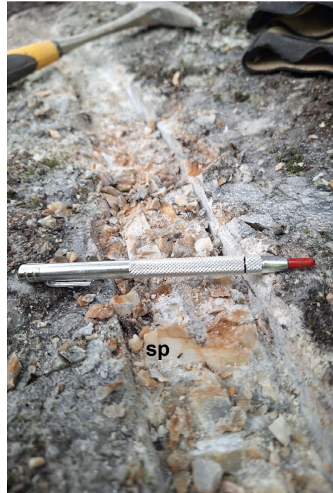
Figure 1: (left) Photograph of diamond cut channel at Orrvik facing south-southeast across strike; and (right) close up of one channel sample interval showing visible spodumene (sp) from channel sample OCSJF06 assaying 2.4% Li 2 O
