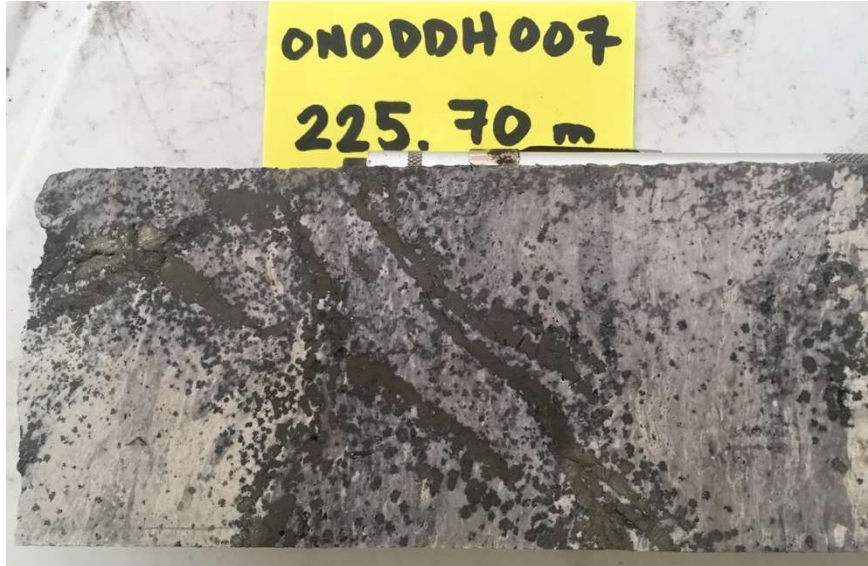
Plate 9 – Altered and mineralized volcanic host rock with up to 7% metallic sulphide in drill hole ONODDH007, HQ core from 225.7 m depth – Ono Island Project, Fiji
