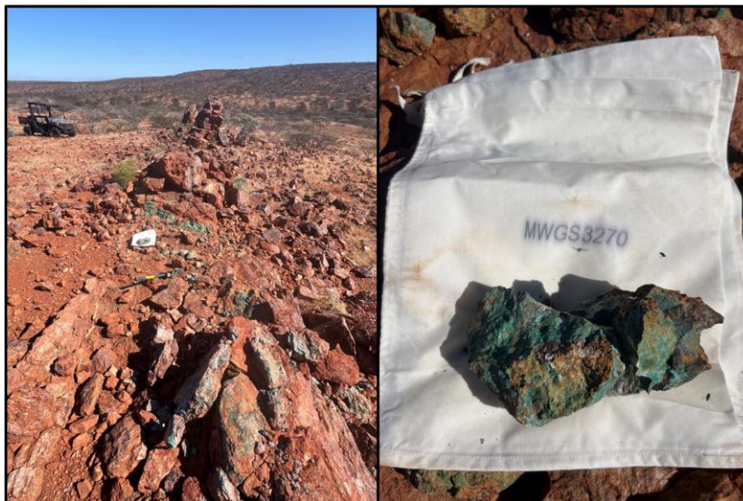
Figure 1: MWGS3270 21.6% Cu surface sampling location looking Northwest mineralisation predominantly occurring as malachite with trace azurite and bornite (see annexure 1).
