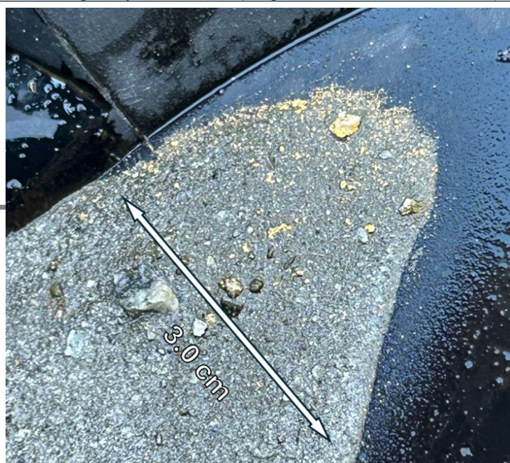
Figure 1: Pan concentrate derived from drill spoil at FOS24RC_056 (23m @ 16.61g/t Au from surface) including the metre panned (1m @ 350g/t Au (from 20m)).
