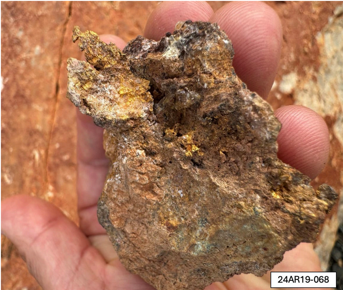
Figure 6. Visible gold in iron oxide quartz vein material located at Titan prospect
