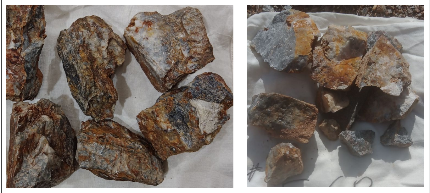
Figure 4: Examples of hand-sized rock chip samples that contain high-grade gold: (LEFT) Mitchells quartz vein breccia containing blue quartz returned 17.92 g/t Au (sample #0658); (RIGHT) Golden Horseshoe blue quartz vein with visible gold returned 12.97 g/t Au (sample #0568).
