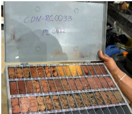
Figure 9: RC drill chips of variegated colour of saponite are stored in chip library
