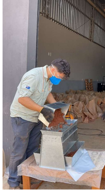
Figure 8: Enova professional geologist sub-sampling by using riffle splitter
