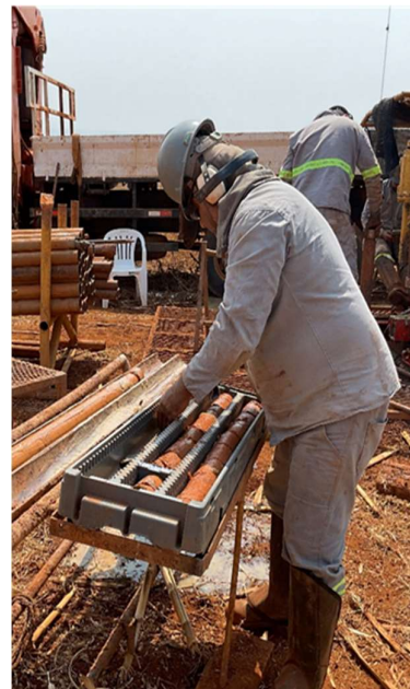
Figure 5: Drill offsider is placing diamond core in core box
