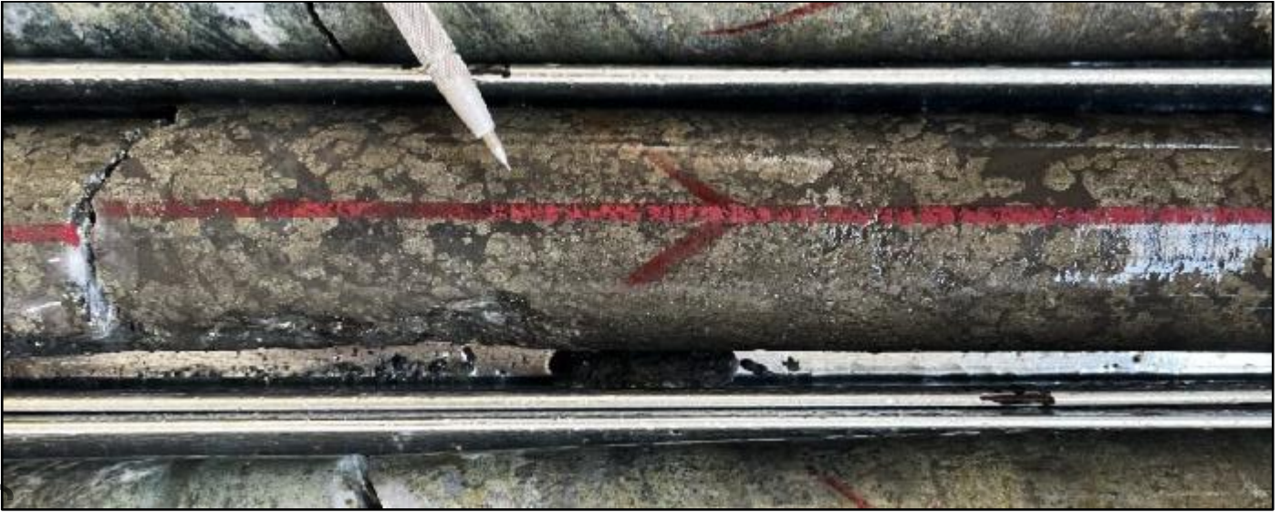
Figure 9. Core photo of semi-massive sulphides with gold mineralisation from 646m in ZRSD24156 – 3.9g/t Au and 2.9g/t Ag
