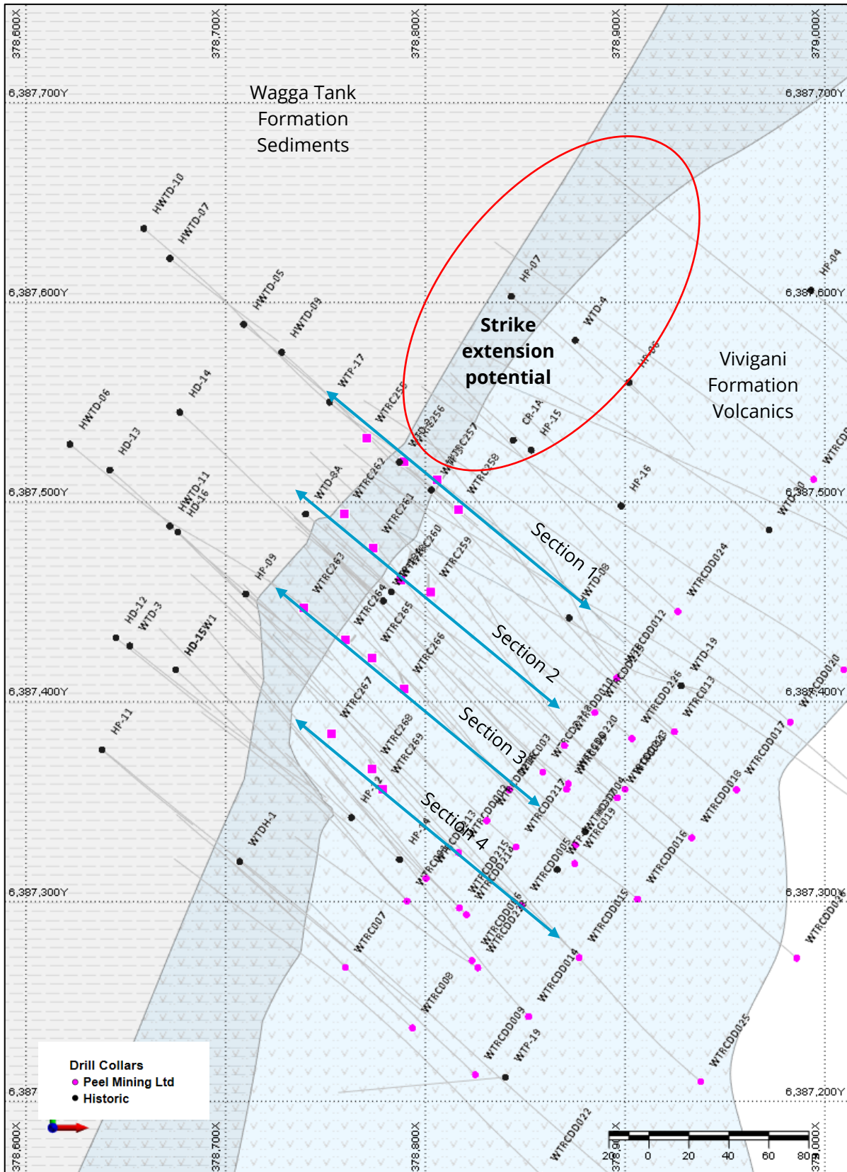
Figure 2 – Wagga Tank Drilling over chargeability ~160m below surface (Magenta = Peel; black = historic)
