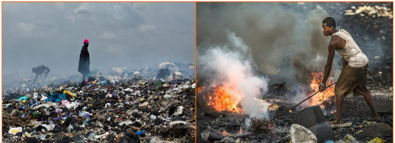
Figure 5: Example of enormous e-waste dump in Agbogbloshie Ghana, Africa. Resident uses fire to burn off plastic, in order to salvage copper wire Source: Hakkens 2016.
