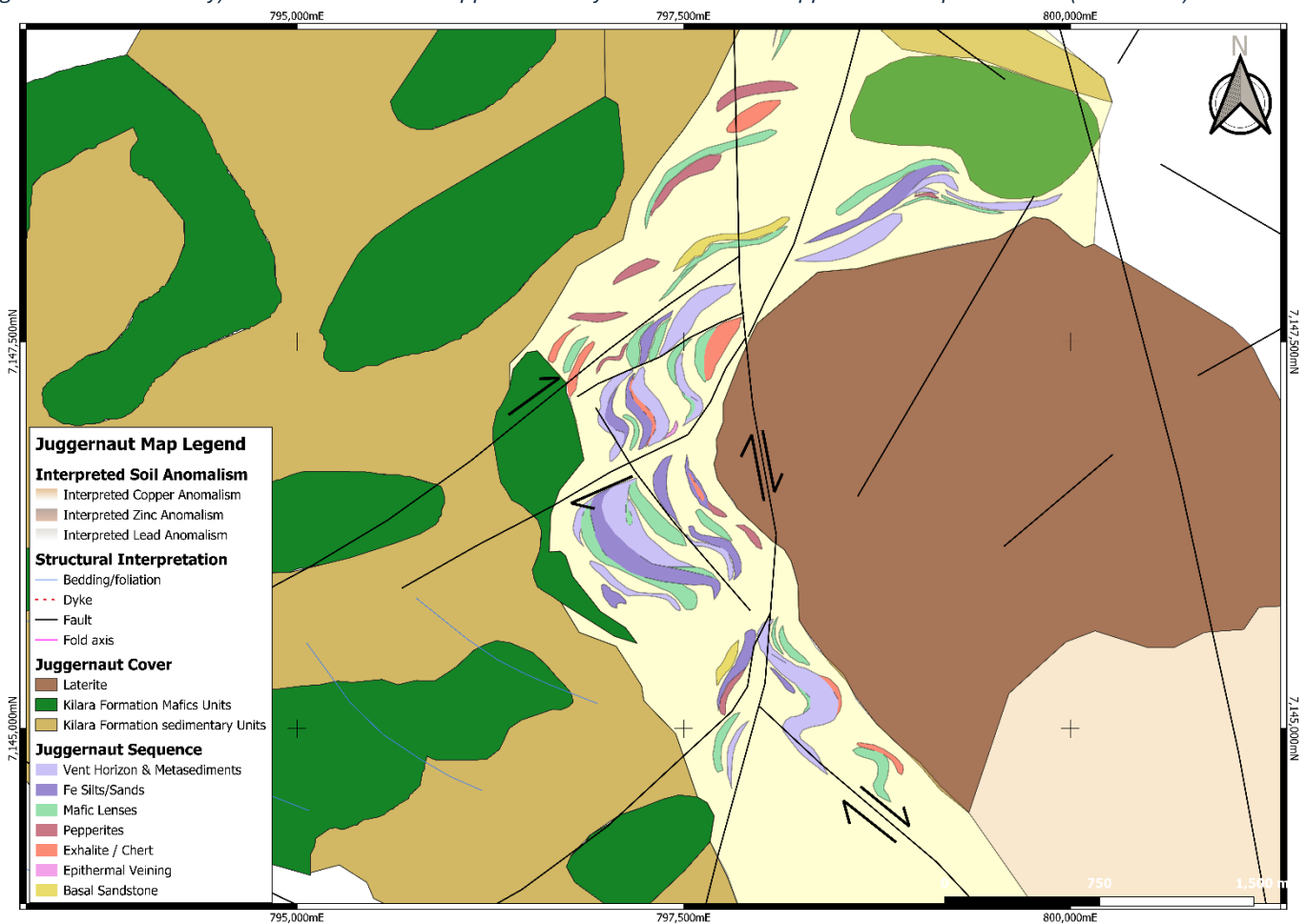
Figure 3: Geological Map of the Juggernaut VHMS Target, overlaid with interpreted levelled copper, zinc, and lead anomalism. The central volcanic and sedimentary rocks are interpreted to be highly prospective for VHMS mineralisation.
