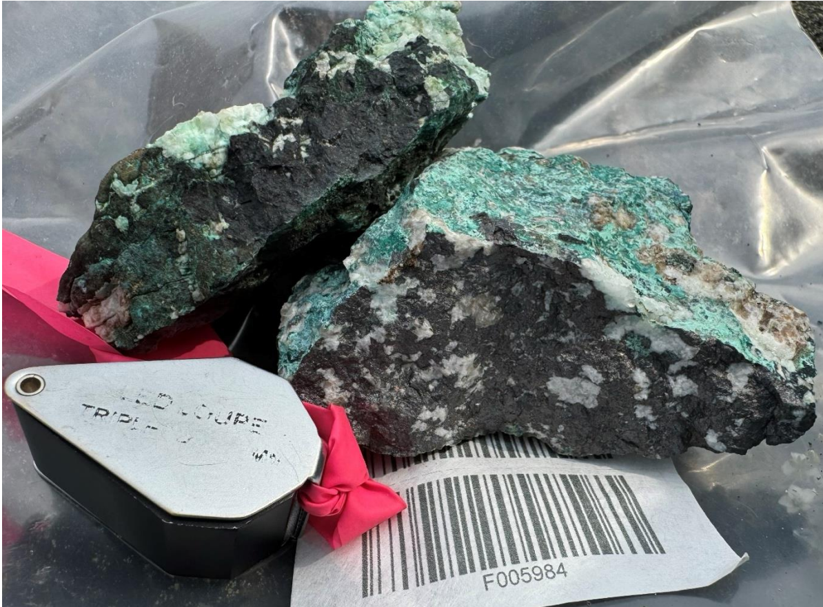
Figure 4: Photograph of sample F005984 which returned 46.07% Cu and 46g/t Ag from the PAT target within the Vision District.
