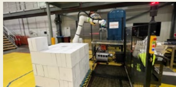
Our Cobot named 'Cooper', is a Fanuc Collaborative Cobot programmed to unload 6 and 12 pack cartons of wine onto the line for relabelling.
