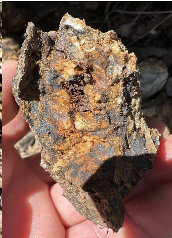
Figure 3 – Silver mineralisation within ferruginous quartz yielding 15.10 g/t Au from sample 3001037
