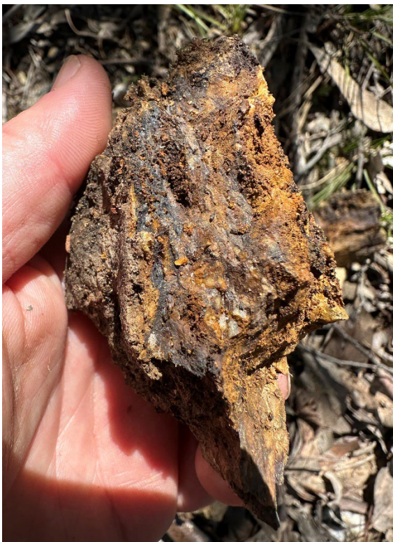
Figure 2 – Gold mineralisation within ferruginous rusty quartz yielding 24 g/t Au & 1.2 g/t Ag from sample 3001038
