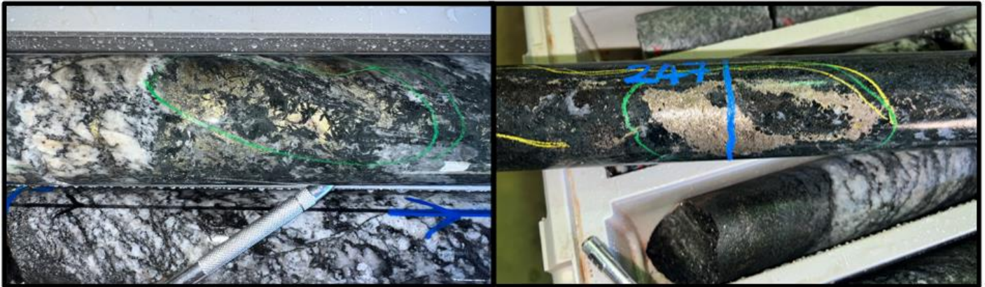
Figure 5: MWDD01 sulphide mineralisation: Pyrite, pyrrhotite & chalcopyrite vein breccia 128.2-128.4m (left). Pyrite, pyrrhotite & chalcopyrite blebby sulphides 246.9-247.1 (right). NQ2 drill core, full sulphide details see annexure 3.
