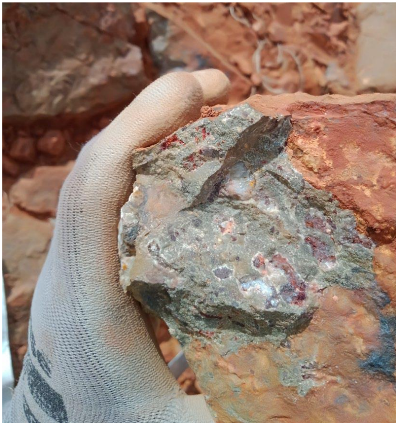
Figure 3: Amygdaloidal intermediate-mafic volcanics identified at the Guinness Prospect area, Mt Maguire Project
