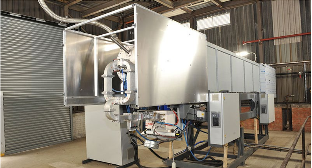
Figure 6: MPI Microwave Rotary Furnace (Source: www.mpiuk.com )
