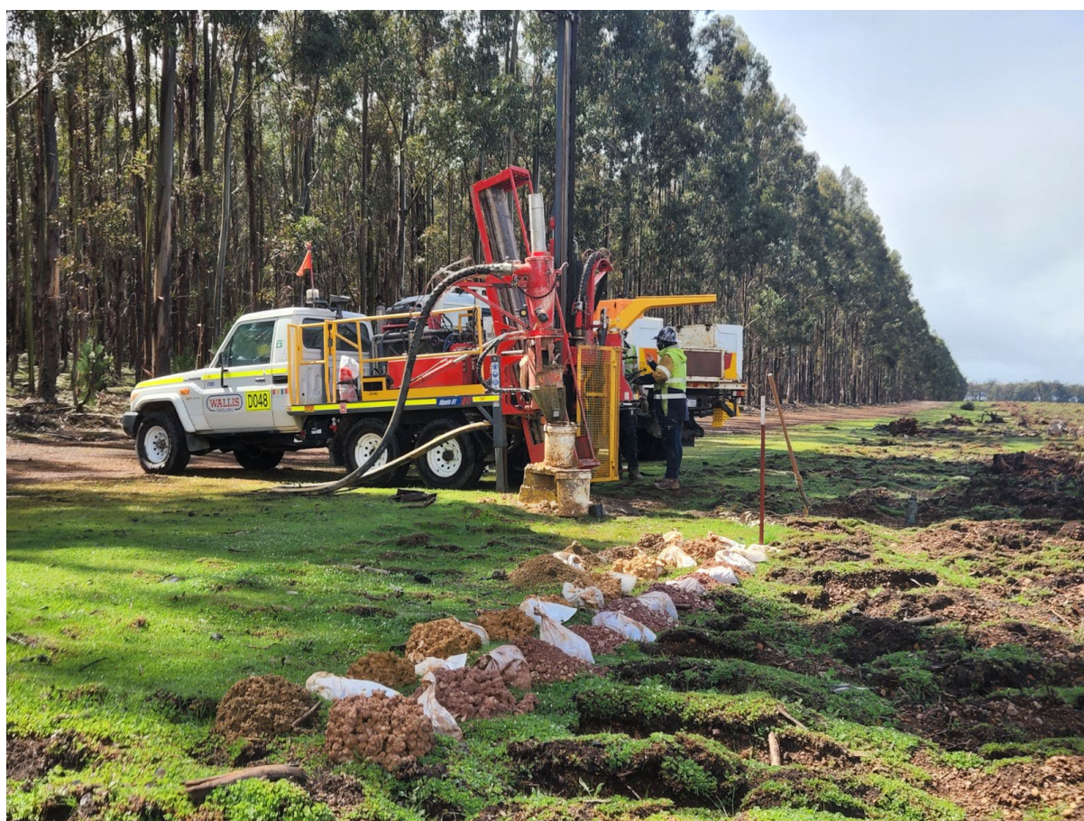
Figure 1. Aircore drilling underway at the Ivar Prospect, WA
