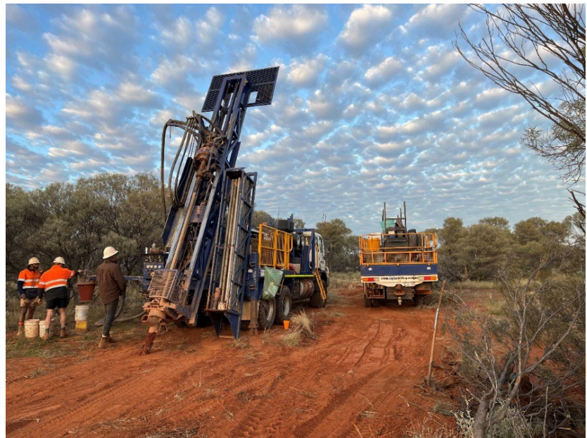
Figure 1. Air-core rig on site at Sword.
