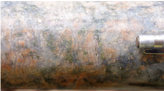
Figure 5. Strongly silicified and altered Briggs granodiorite with micro-UST textures and extensive copper sulphides.
