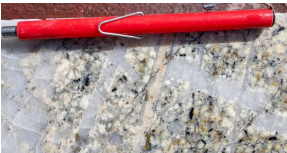
Figure 3. Intensely altered porphyritic granodiorite with quartz-feldspar stockwork veins. Hole BD019003, 257.7m down-hole depth from a sample assaying 0.18% Cu.
