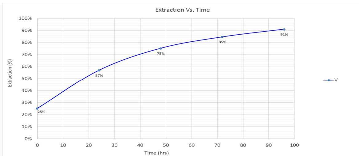
**Figure 5: Vanadium extraction from Magnetite concentrate over leachate time**
