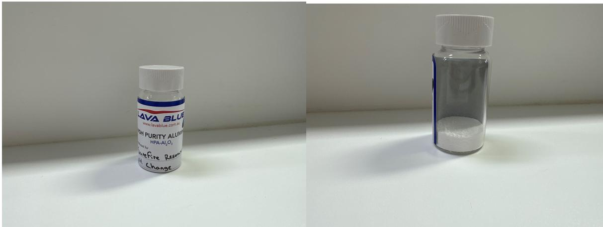
**Plates 1,2: Some of the first 4N 9.99% HPA generated by Lava Blue from the Company’s Victory Bore deposit**
