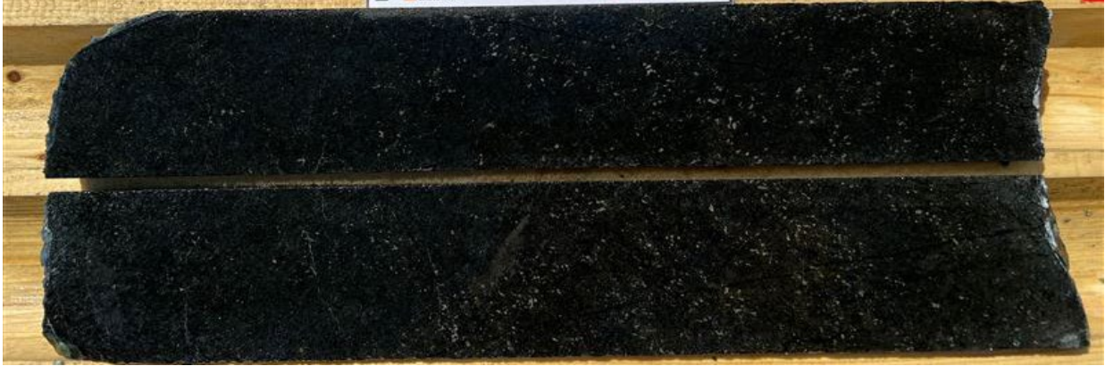
Figure 8: DDED23-131 interstitial to disseminated sulphide mineralisation
