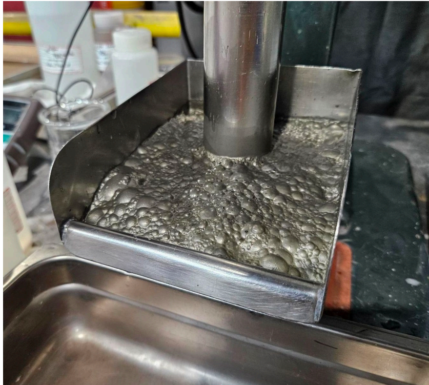
Figure 14: 3rd cleaner sulphide concentrate assaying 29.1% nickel
